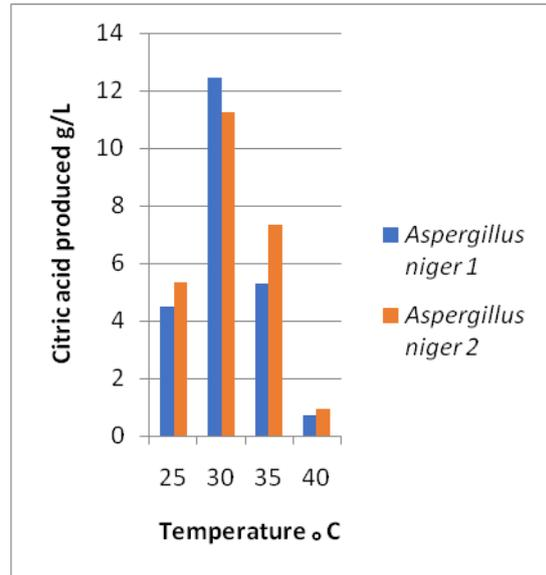
Fig 4: Effect of different temperatures on citric acid production by *A. niger 1* and *A. niger 2*
